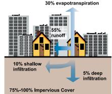
Relationship between impervious cover and surface runoff. Impervious cover in a watershed results in increased surface runnoff. As little as 10 percent impervious cover in a watershed can result in stream degradation.
